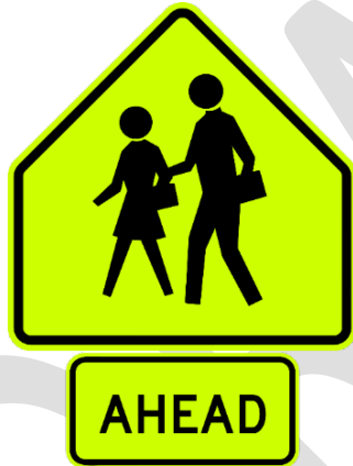
Figure 57: School Advanced Warning Assembly - S1-1 w/ W16-9P
