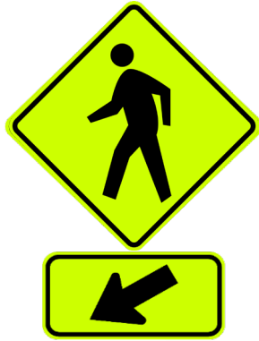
Figure 55: W11-2 sign with W16-7L left diagonal arrow
